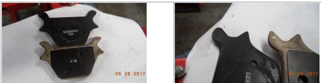
These 2 different brand of brakes look very similar. 11) The OEM pad on right has sharper contours 12)
