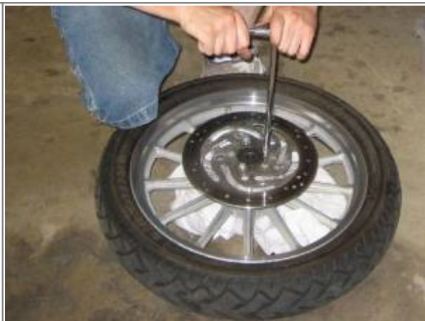
Remove 5 Torx bolts (T40) holding brake rotor on. An impact wrench was used to loosen the bolts. 8)
