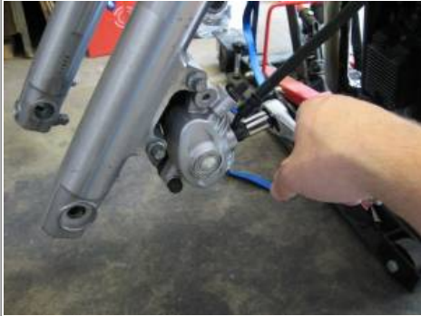
Brake line stuffed into an old oil bottle and bungee'd out of the way 6)
