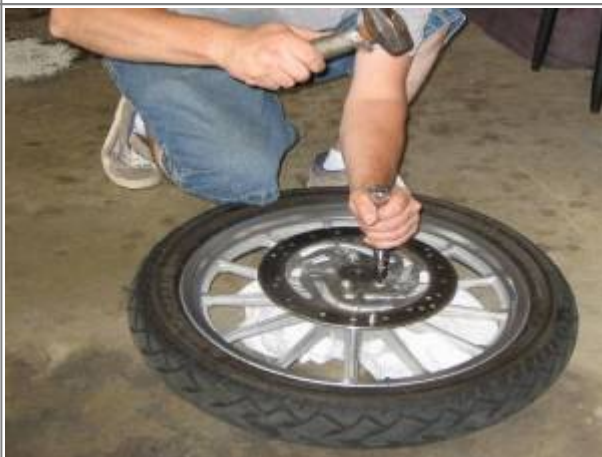
Remove 5 Torx bolts (T40) holding brake rotor on. An impact wrench was used to loosen the bolts. 8)
