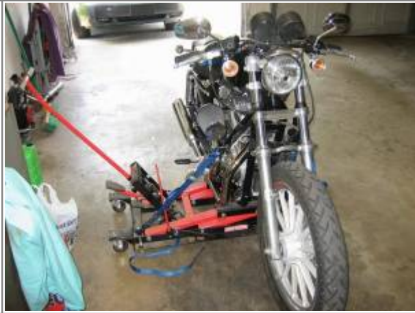
Remove old caliper, pull axle out while catching the spacers and remove the tire 5)
