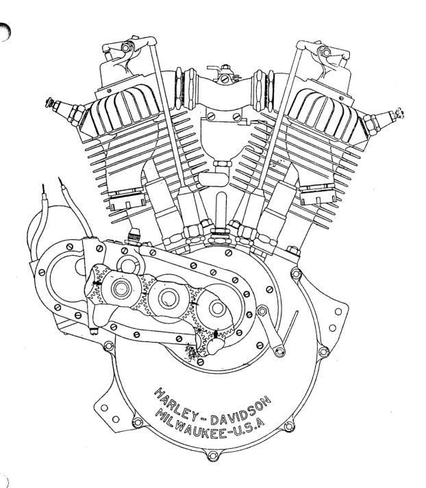
7-32 inch to 9-32 inch before top center on the compression stroke. Remove the bakelite distributor cap and the high tension distributor segment. Remove the hexagon nut clamping the circuit breaker cam, advance the circuit breaker as far as it will go by pushing it forward and moving the cam on the shaft in the direction that it runs so that the circuit breaker points are just starting to break contact. Then tighten the cam clamp nut securely.
