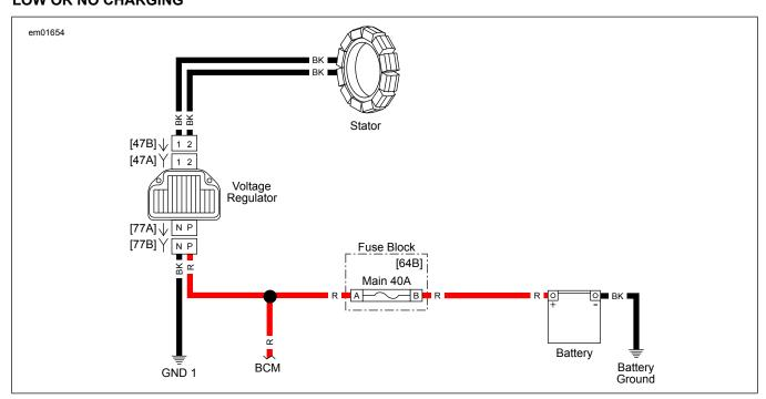
Figure 1. Charging System Circuit
