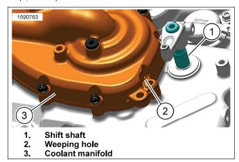
Figure 1. Weeping Hole (Bolt remove for clarity)
