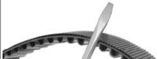
Figure 1. Improper Handling of Drive Belt During Rear Wheel Removal
