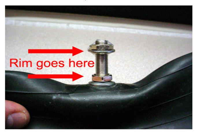
The washer is **not** used on the Profile rim (Part # 43570-06) as this rim has a smaller valve stem hole.
