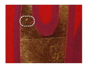
A burnish void occurs when a sheet is burnished and a spot is slightly lower than the rest of the surface. This low spot does not become burnished and remains brighter or shinier than the surrounding area.
