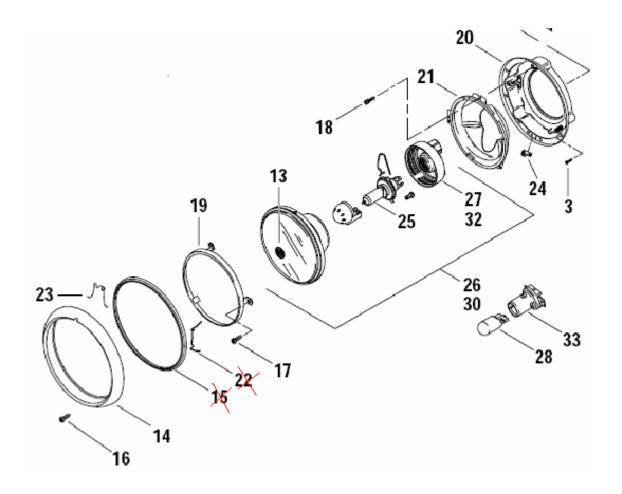
One other less visible change also took place due to a supplier change for the headlamp assembly used in production. The retaining ring, Item 19 above, will appear to protrude a bit more and it will have a duller finish than the older version.
