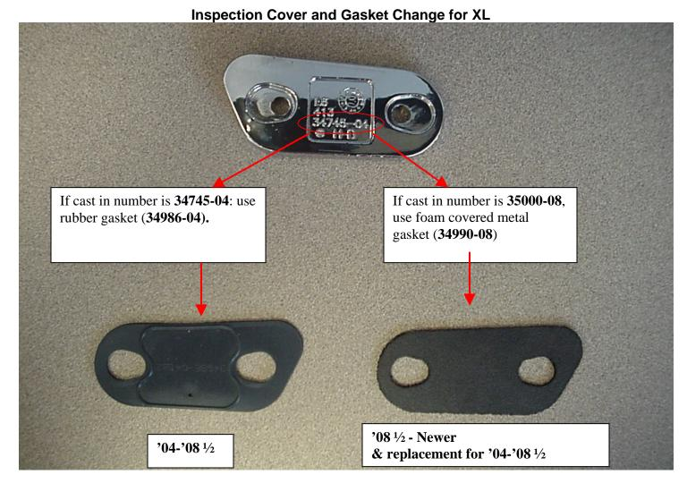
Starting May 5, 2008, All Sportster models received a new inspection cover and gasket as a running change. These new covers and gaskets do retro-fit back to 2004; however, the previous style -04 covers require the use of the previous style rubber gaskets, and the new style -08 covers must be installed with the new style foam gaskets. These parts can be identified visually (see figure above).
