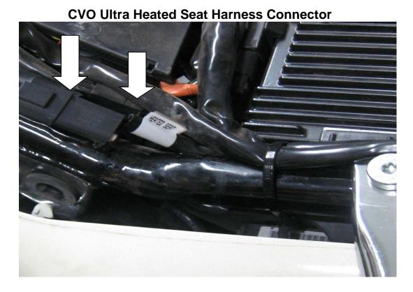
Remember, on earlier bikes the two connectors are not labeled. Please be sure to identify the correct connector for the heated seat when installing. You will notice that the heated seat connector has two wires only, O/R and BK. It is always a best practice to verify that the heated seat works after any service that requires the seat to be removed.
