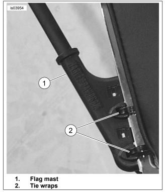
Figure 1. Exterior View of Installed Flag Mast
