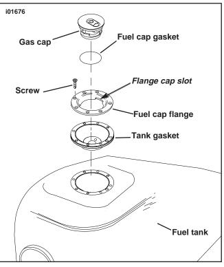
Figure 1. Gas Cap Assembly Installation
