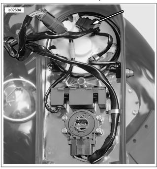
Figure 6. Speedometer Connector [39] (2004 FXST shown)
