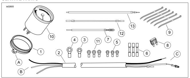
Figure 7. Service Parts, Mini-Tach Gauge Kit
