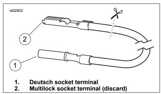
Figure 3. Cut Multilock Terminal From Adapter Lead
