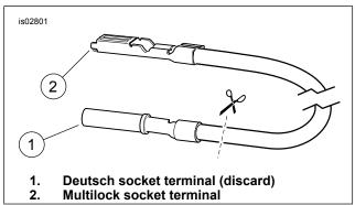
Figure 4. Cut Deutsch Terminal From Adapter Lead
