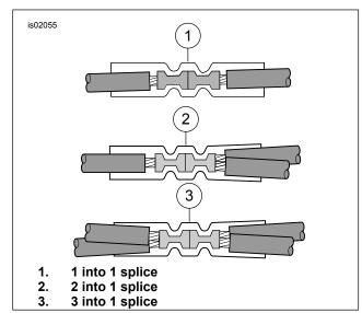
Figure 1. Splice Configurations
