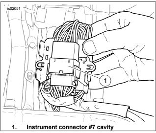
Figure 5. Instrument Lights Connector [20] (2003 XL Custom shown)
