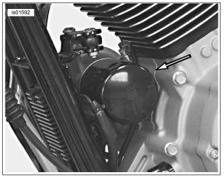
Figure 1. Spin-On Oil Filter (Sportster Evolution Engine)
