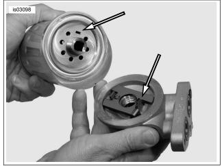
Figure 3. Oil Filter Housing/Anti-Rotation Device Alignment
