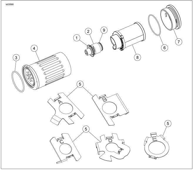
Figure 5. Service Parts: Definitive5 Filtration System Kits
