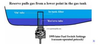
Starting in 1992, when there was an option for a 3.25gal Sportster tank, the petcock specified was a new, vacuum-operated design. It had an automatic shutoff function that used a vacuum hose connected to the carburetor (tee'd off the hose to the VOES) to operate a diaphragm in the petcock. This diaphragm had a short plug that protruded into the fuel flow cavity, and held there by a spring, to prevent fuel flow until there was enough vacuum to pull the diaphragm/plug out of the cavity.
