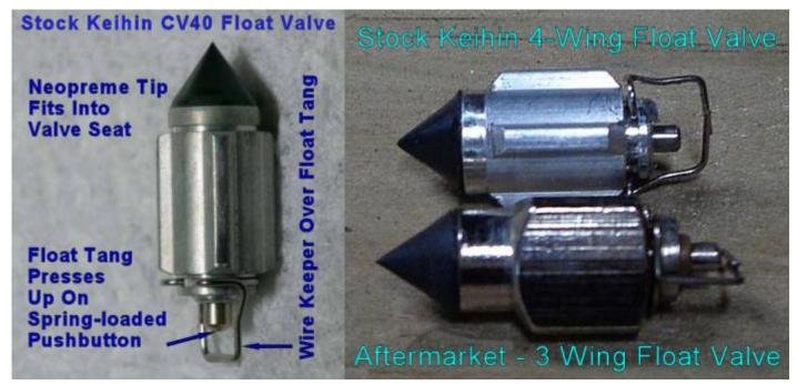
In This XLForum Thread there is a discussion of the float bowl overflowing and the possibility that it is caused by aftermarket float valves that are not of the proper design. 10)
