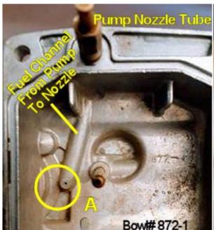
1989-2003 Float Bowls have a fuel supply channel from the Accelerator Pump to the Pump Nozzle Tube. A bleed hole (A) in that channel is used to receive fuel from the bowl into the pump reservoir. The same channel is used to send the pumped fuel to the Pump Nozzle and the bleed hole relieves excess pressure.
