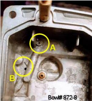
2004-2006 Float Bowls uses a similar fuel channel between the Accelerator Pump and the Pump Nozzle Tube. Because the check valve was relocated into the AP body, this version uses a hole (B) in the bowl, separate from the fuel supply channel, to receive fuel into the check valve & to the pump reservoir. 29
