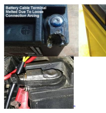
As you can see in the pictures above, if the connections are not tight even the posts can melt due to high current arcing. The operational vibrations often loosen bolts of all sorts on the bike, including the battery cables. In addition to tightening the bolts, you can physically restrain the connectors with a zip tie around the battery post. With proper placement, even the rubber boots can be put back in place.
