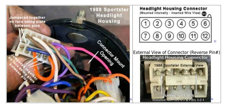
1986-1990 Wiring of the Headlight Housing Connector
