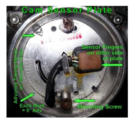
Moving the Cam Sensor Plate Clockwise (CW) will increase the Advance Before TDC. Moving the plate Counterclockwise (CCW) will retard (or reduce) the Advance Before TDC. TAKE NOTE that each timing mark on the plate (long-to-short) is equal to changing the ignition timing by about 5°. Move the plate <u>VERY LITTLE</u> to make adjustments. <sup>13)</sup>
