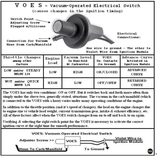
See the explanation of manifold absolute pressure -vs- vacuum gauge readings in the REFerence section on the'Ignition Modules - Aftermarket' page:
