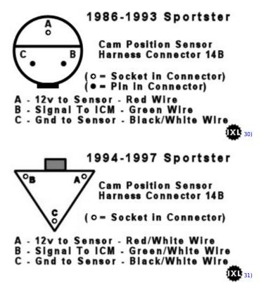
(Note: the 1998-2003 Sport model uses the same CPS & Connector as the 1994-1997 models. The slotted rotor cup is different on the Sport models, having additional slots to allow for the single-fire ignition. Note
