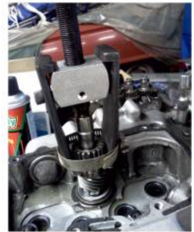
FLYWHEEL PINION GEAR - PULLER Get the Harbor Freight gear puller #66868 and grind the end tips a bit to get them thinner. Remove the oil pump first and use a hose clamp on the end as shown. Works great! http://www.harborfreight.com/catermotive/puller-puller-66868.html
