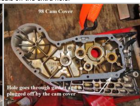
2000-up gasket seals off the extra hole. 25)
