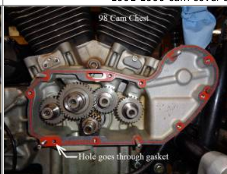
2000-up gasket seals off the extra hole. 25)
