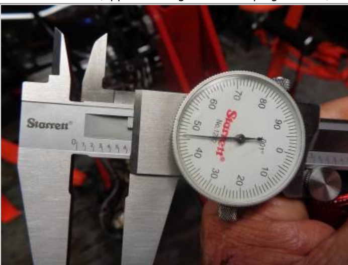
Measured from the case outside surface to the app. end of the case threads (app. 1/4" longer than the plug threads). 7)
