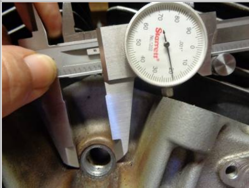
Notice the plug doesn't go all the way into the end of the case threads 4)
