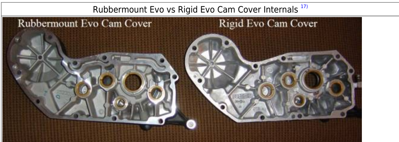
Both have been chopped on the outside but the gearcase perimeter is intact on them for reference.
