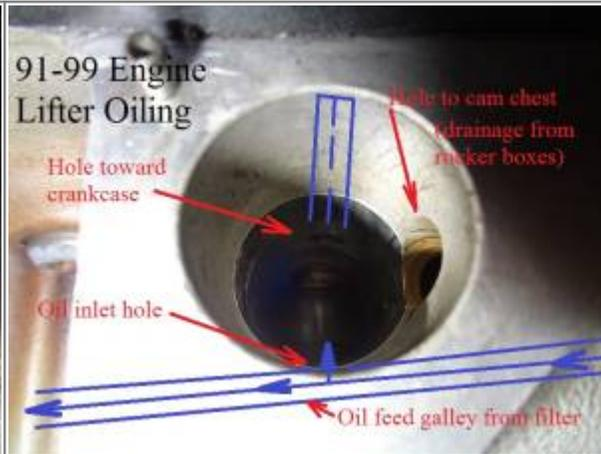
A look inside the oiling holes in the lifter bore on a 91-99 case. Notice the capped hole toward the case in the third pic. <sup>41)</sup>
