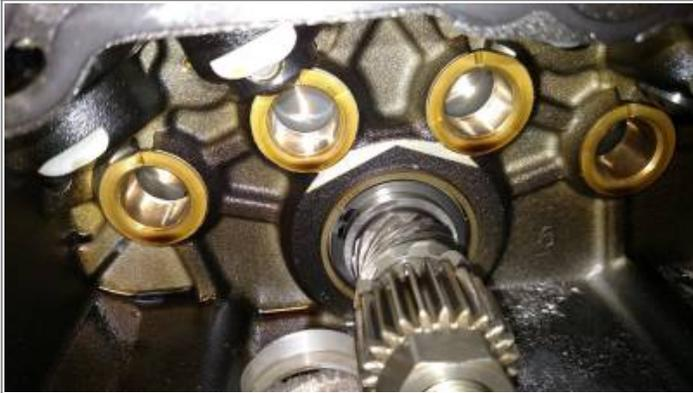
2010 1200X Inner Cam Bushings (broken teeth on oil pump gear)<sup>24)</sup>
