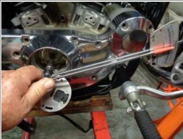
Installing timing cup bolt on a 98 1200S <sup>73)</sup>
