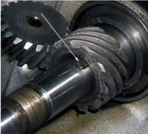
The pinion gear is located by the little nub of the oil pump drive key that you see sticking out. With high valve spring pressures, this nub often shears off, sending pistons crashing into valves. Avoid this issue by torquing the pinion nut to 70lb-ft. Be sure to use Loctite red on the threads per the manual.
