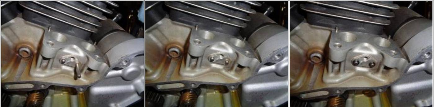
Then install the plate and torque to 80-110 in lbs. <sup>47)</sup>
