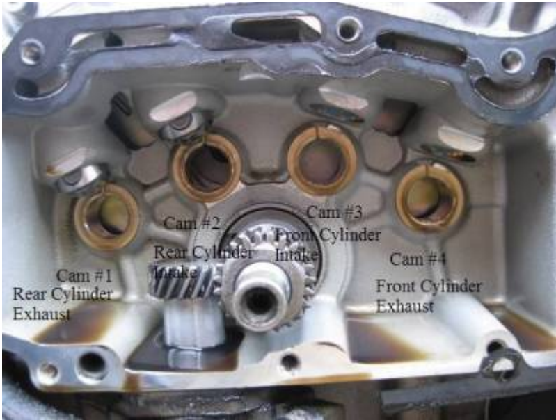
Cam hole identification in the gearcase: 9)
