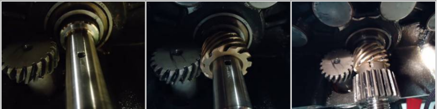
Be in mind of the woodruff key location in the pinion gear slot. 29)
