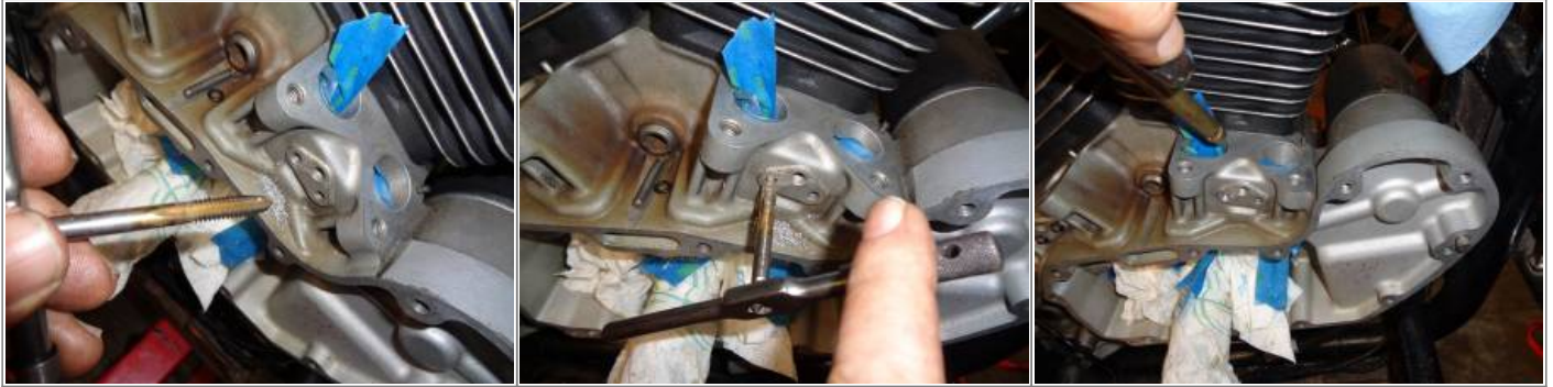
You can use a small inspection camera to check the oiling holes for aluminum shavings. 23) This is the new extended pin hole. 24)
