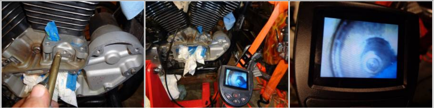
This is the oil feed hole in the bore. 25) The blind hole on the inside of the bore got splashed during blowdown. 26) A straw into the air gun placed in this hole removed the chips. 27)
