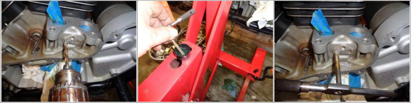
Remove the tap periodically, clean the shavings off of it, oil it and run it back in to continue threading. Blow the chips out with compressed air. 22)
