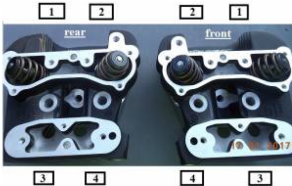
Head Bolt Removal and Installation Torque Sequence
