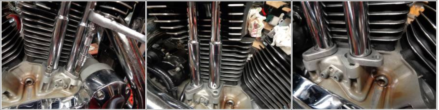
The short Allen adapter and extension brings the wrench to the smaller OD area of the tube. 2)
