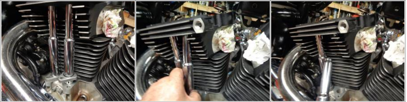
There is enough room to pick up on it and then pull the bottom out to clear the lifter block and then down to remove it from the head. 3)
