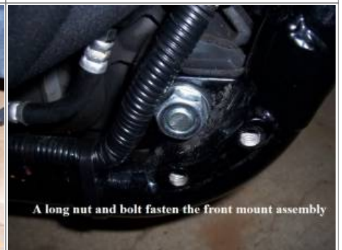
A long nut and bolt holds the front assembly. 31)
