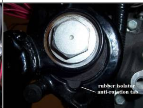
Built in anti-rotation tabs. 66)
