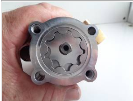
Feed Gerotors Installed 7)
