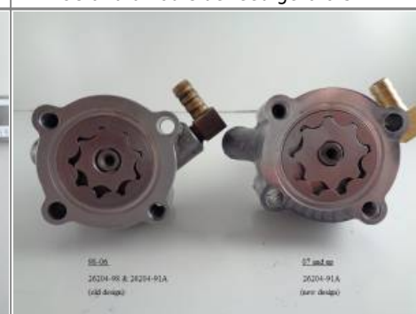
98 and 07 feed gerotors installed 26)
