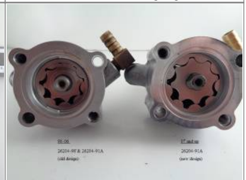
98 and 07 scavenger gerotors installed 15)
