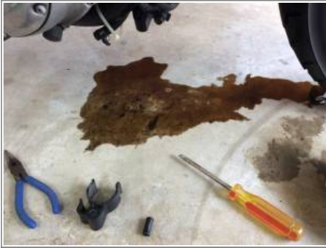
Broken oil drain clamp 3)
