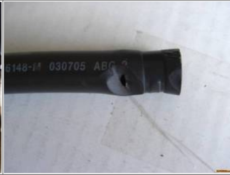
Drain hose hole worn in by the motor mount. 4)
