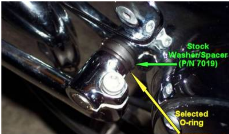
2006 Sportster - added O-ring (5/8 OD x 1/2" ID x 1/8" thick)
