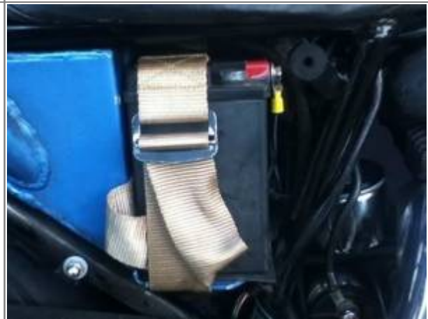
Possible temp fix for missing bracket 71)
