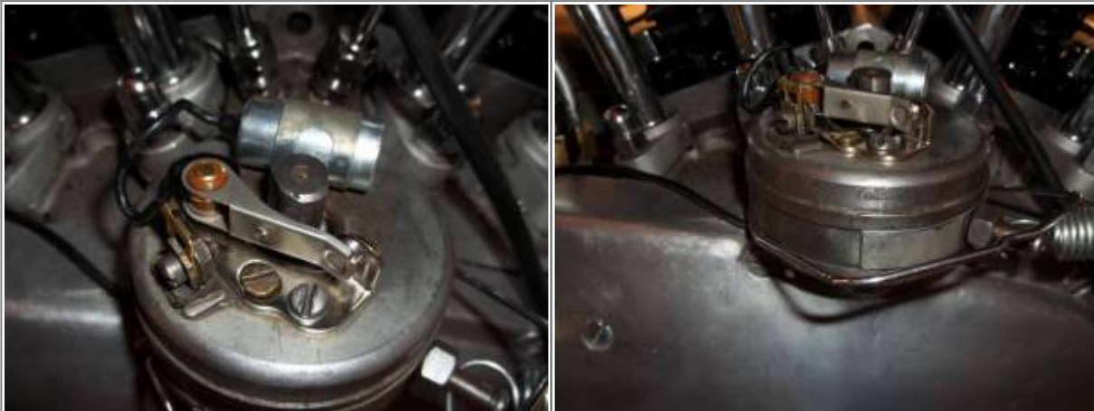
Single Point Circuit Breaker on a 57 XL 8)
