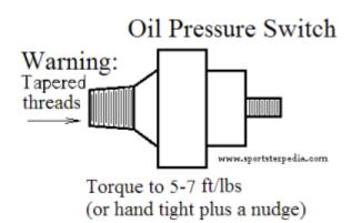
**Caution**: DO NOT tighten the oil pressure switch too tight.
