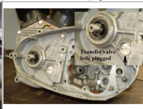
Transfer valve removed, plug installed. 7)
