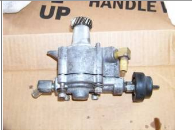
Rubber boot pulled over the oil pressure switch 58)
