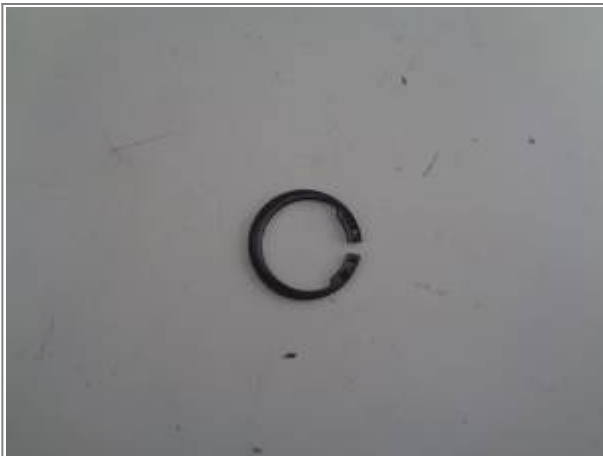
Gear shaft retaining ring (26497-75) 8)
