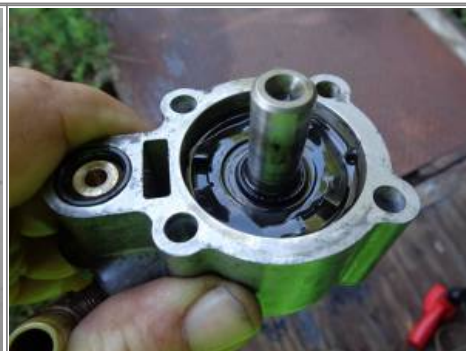
Spring washer installed 34)
