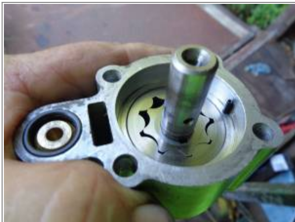
77-E83 return gerotors installed position 48)
