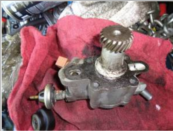
Oil pressure switch mounted to the oil pump 57)
