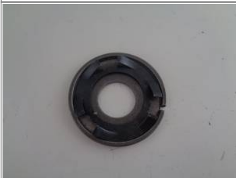
The spring washer fits inside the inner plate. Fingers face toward the feed gears / cover. 33)
