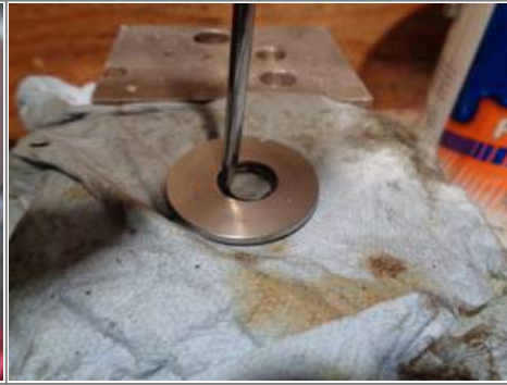
Outer seal (12036A) installed 30)
