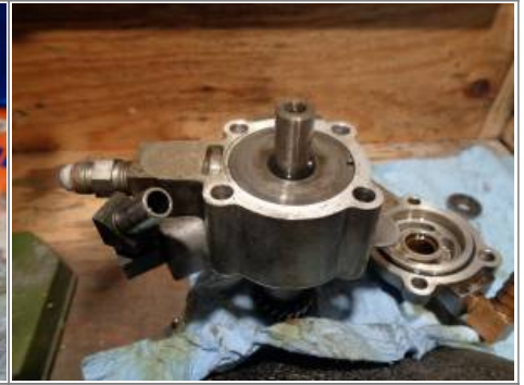
Outer seal (12036A) installed position on 86 pump. 31)
