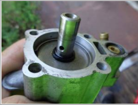
Outer seal (12036) installed 29)
