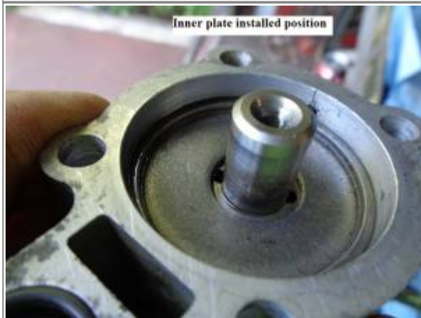
Inner separator plate installed position. (pump upside down) 17)
