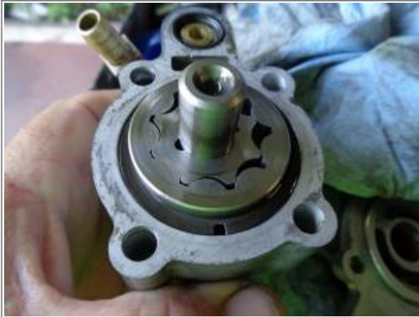
77-E83 feed gerotors installed position 45)
