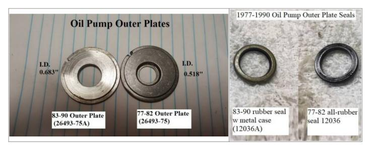
The damage below was caused by using the wrong seal (83-90 seal with the metal shell) in the 77-82 outer plate with the counterbored seal hole. The plates (when installed) are very close together and the 83-90 seal doesn't sink down flush to the plate. This puts added resistance to the pump turning and as seen below, the seal will grind away at the counterbore and/or lock up the pump.
