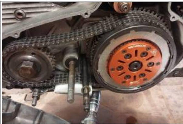
77 XLH with 86-90 Primary Chain Tensioner & Spring (40019-86) 1)
