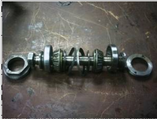
1980 Swingarm bolt assembly 3) The best way to get the bearing races in and out is with a large nut and bolt, like 1/2" UNF, and some large flat washers
