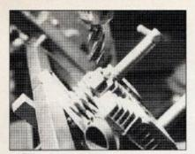
A 7/8-inch milling tool is then used to bore the clearance hole that will accommodate the spark plug socket. This hole must be bored until a flat surface is obtained at the bottom of the hole in the solid, non-finned part of the head.
