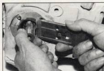
32 Ditto for the mainshaft end play (.003" - .009"). However, you must also press against the clutch gear so that the door bearing seats against the retaining ring in the door as you take your measurements.
