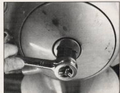
5 The old 'Chevy tool' is used to remove the clutch adjuster plug.
