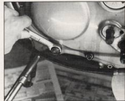
4 Next, take off the nut on the end of the chain tensioner stud.
