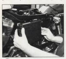
After servicing and fully charging the battery, reinstall it in the motorcycle. Reconnect the positive cable first, then the negative (ground). Be sure the vent tube, if applicable, is properly positioned.
