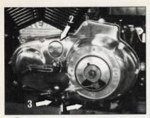
Change the primary fluid. The drain plug (see arrow 1) is on the underside of the primary. Also check the chain tension through the inspection cover (see arrow 2). The chain tension is adjusted with an adjusting bolt (see arrow 3) on the underside of primary.
