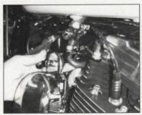
Use your fingers and eyes to look for fuel system leaks. If your finger's wet, you have a leak. Also, bend all hoses sharply and look on the outside of the bend for cracks, a sure sign of dry rot.
