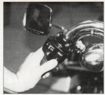
With the battery fully charged, check that all electrical equipment and switches, including headlight, turn signals, brake light and horn are working correctly.
