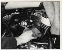
After you remove the air cleaner's cover, clean it and the backplate with a clean rag. If the filter element is damaged, replace it. If it looks suitable, wash the element in soapy water.
