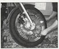
Inspect the front and rear tires for excessive or uneven wear.
