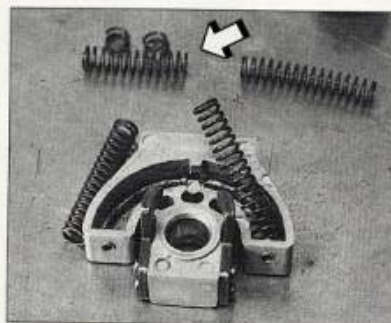
12 More broken stuff, this time a pawl carrier spring (see arrow). The new ones are sticking out of the shifter pawl. I can't believe this bike was still shifting gears!
