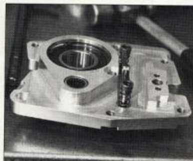
15 This is Zipper's billet aluminum door. Forged billet aluminum is much more resistant to wear than a cast aluminum one. This, combined with the larger surface area of the Zipper's double row bearing, prevents the wear common to the stock door.
