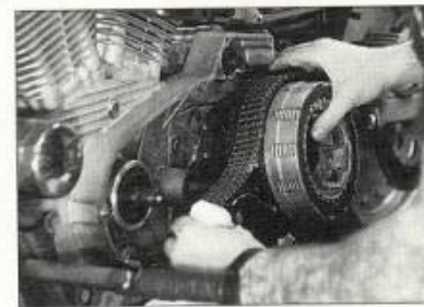
6 After removing the engine sprocket, Rich can remove the entire primary drive and clutch at the same time.
