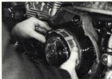
26 It's time to install the primary drive. Rich gives the clutch shell a hearty shake and states that the whole assembly is much tighter on the shaft than it was with the stock access door.
