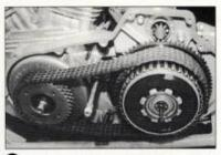
You can now remove the outer primary screws in a sequential pattern. Then remove the primary cover from the engine case and carefully set it off to the side. Remove and discard the primary cover gasket.
