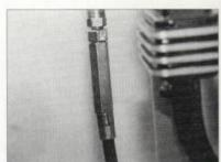
B Return to the cable adjuster and remove the slack from the cable. Then loosen the adjuster until you have 1/16" to 1/8" of free play at the lever. Now lock the jam nut and slide the adjuster's boot back into position.
