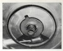
Reinstall the retaining spring into the hex adjusting nut.
