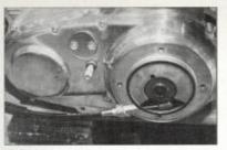
Install the outer primary cover using a fresh gasket. Torque the screws down to 80-110 in-lb. Refill the primary case with 24 ounces of primary lubricant. Install the cable actuator, hex nut, and a new O-ring.
