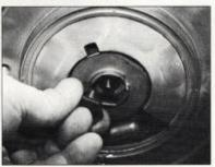
Turn the clutch adjusting screw clockwise until the hex nut can be removed. Place it with the other parts.
