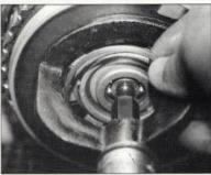
After removing the outer snap ring, nut, and spring compression tool, you can then remove the outer and inner clutch spring seat, clutch spring, and pressure plate.
