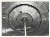
Turn the clutch adjusting screw counterclockwise until the free play has been removed from the screw, then back it off 1/8 turn and lock down the jam nut.
