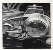
Remove the primary drain plug from the bottom of the primary cover. Drain the primary oil into a suitable container. Dispose of it safely after the job is finished.
