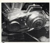
Remove the footpeg and shifter lever. Then loosen the locknut and unscrew the chain adjuster to relax the primary chain's tension. Remove the derby cover from the outer primary and set it aside.
