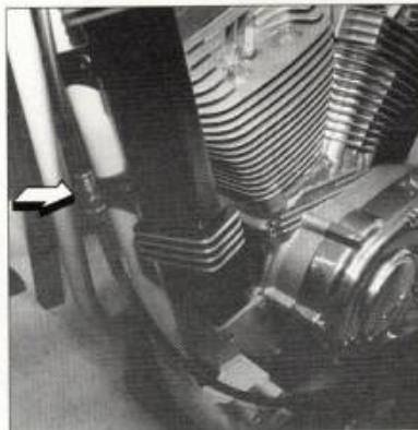
2 Slide the protective rubber boot away from the adjustment turnbuckle in the middle of the clutch cable and adjust the turnbuckle to its loosest position.
