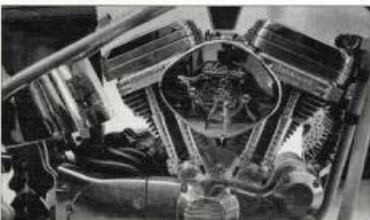
29 Next, install the Edelbrock intake manifold to the head assemblies. Then install the new QwikSilver carb assembly, cables, and air cleaner as per the instructions and you're good to go.
