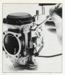
3 Remove the four screws on top of the carb and the big screw on the cable guide in order to remove the carb's top, spring, and slide.
