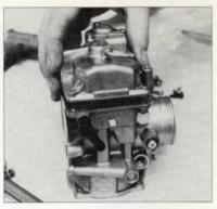
Reinstall float bowl. If your bowl gasket looks questionable, replace it. Be sure the accelerator pump rod and boot are seated in the pump housing before tightening the float bowl screws. You're now finished with the bottom of the carb.
