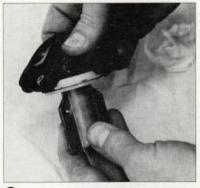
off the stock slide. Make sure you remember which is the "up" side of the diaphragm. Install the diaphragm onto the Thunderslide kit's black plastic slide, sandwiching it between the snap-on plastic washers.
