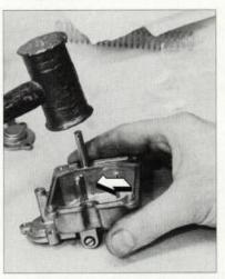
(3) Drop the Thunderslide check ball and spring into the enlarged hole. Align the Thunderslide nozzle so the squirt hole faces the brass tube in the center of the bowl (see arrow). Tap nozzle lightly into place using a soft or brass hammer.
