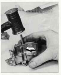
® Drop the Thunderslide check ball and spring into the enlarged hole. Align the Thunderslide nozzle so the squirt hole faces the brass tube in the center of the bowl (see arrow). Tap nozzle lightly into place using a soft or brass hammer.
