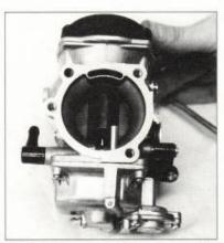
The Thunderslide's black plastic slide and big accelerator pump nozzle are plainly visible on this assembled CV. After you've reinstalled the carb on your Sportster, you're ready to start kickin' butt and takin' names.
