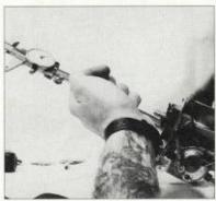
Measure the float level and make sure it is correct. Read your service manual for how to do this and the required specifications.
