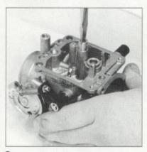
Install the Thunderslide emulsion tube. Select a main jet (the instructions are very helpful about how to do that) and screw it into the emulsion tube.
