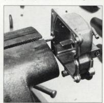
Clamp the nozzle in a vise, and twist the bowl to remove the nozzle. Also remove the stock spring and check ball that live under the nozzle.
