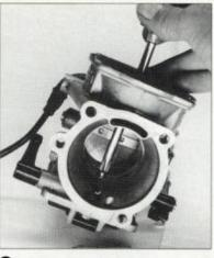
Onn't lose the small silver section of the emulsion tube that we're pointing to with the screwdriver. It must remain in place to be used with the Thunderslide emulsion tube.
