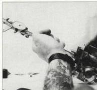
Measure the float level and make sure it is correct. Read your service manual for how to do this and the required specifications.
