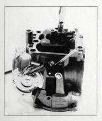
Remove the float bowl, then remove the stock main jet and brass emulsion tube. Sometimes they come out together.
