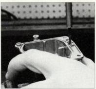
Using the shouldered drill provided, enlarge the pump nozzle hole until the shoulder hits the edge of the bowl. Be sure to clean the hole thoroughly with carb cleaner to remove all the aluminum shavings.
