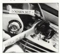
Installation is much easier with the carb off the bike. When loosening the big steel nut behind the choke nut bracket, remember to turn the nut clockwise, or the plastic threads will be destroyed.
