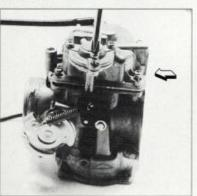
4 Flip the carb over and remove the four screws at the corners of the float bowl (see arrow). Do not remove the screws we're taking out unless you want to inspect the guts of the accelerator pump.
