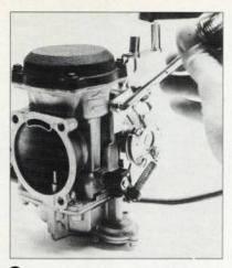
Remove the four screws on top of the carb and the big screw on the cable guide in order to remove the carb's top, spring, and slide.
