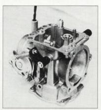
3 Using the supplied drill bit, carefully pierce the aluminum plug covering the idle mix screw. Remove the pierced plug with the supplied screw.
