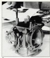
• Gently bottom the idle mix screw and then turn it out 1 1/2 turns. Note: contrary to what the directions say, many 1200s are happiest with a 45 low speed jet, especially if they have aftermarket pipes. A good starting point for this jet is 1 1/2 turns. If you have a smaller low speed jet, this may be a good time to replace it.
