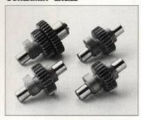
Harley-Davidson offers a bolt-in alternative to the stock camshaft in your XL Evolution engine. These camshafts are designed and engineered specifically for use with the stock production hydraulic lifters, springs, and pushrods. These camshaft profiles offer longer durations on both the intake and exhaust for greater peak torque and improved horsepower from 2500-6000 RPM. The #25628-89 camshafts fit 1986-90 Evo four-speed models and the #25648-91 cams fit 1991 and later five-speed models.
